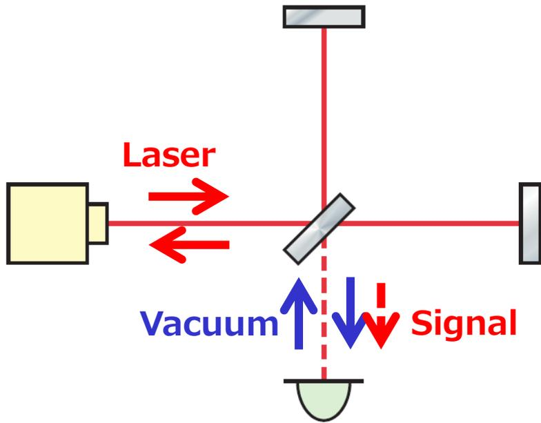
Vacuum field consists of amplitude and phase fluctuations.
