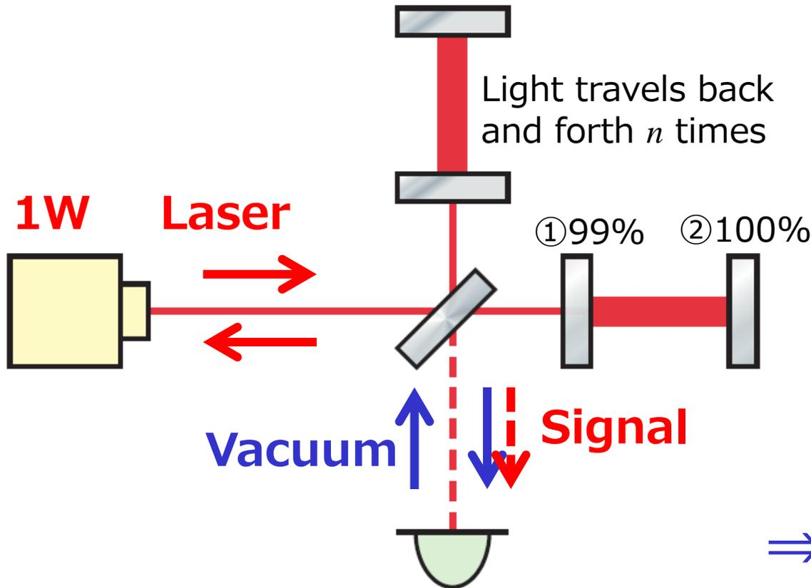
With a cavity to circulate light 400 times, both  $\sqrt{N}$  and  $\Delta L$  increase by 400
