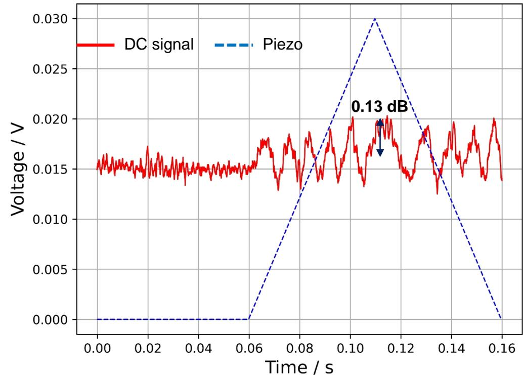
**Dithering the arm at 1kHz and sweeping the pump phase, we found a 0.13dB oscillation of output of a lock-in amplifier at dark port.**
