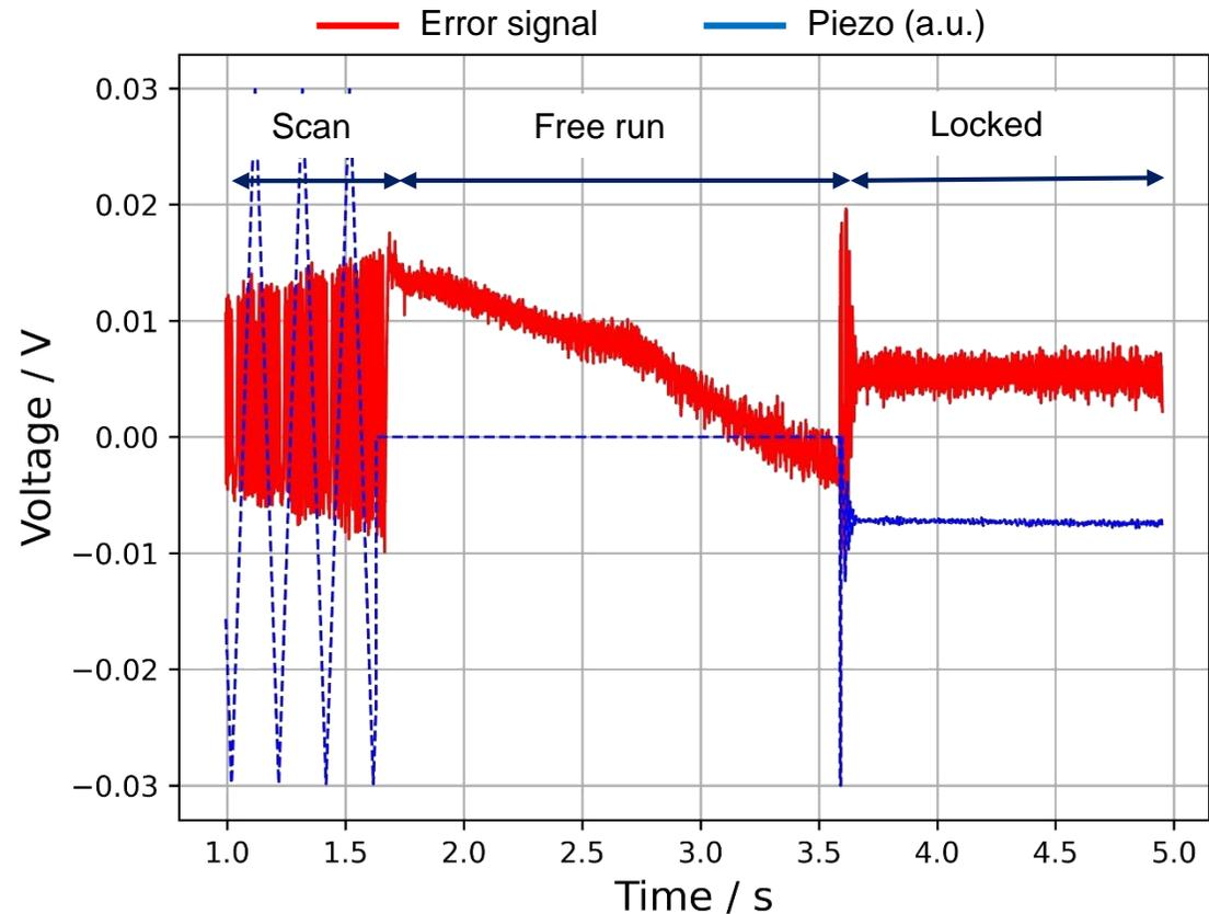
**With the coherent control, the OPA phase is locked to the amplitude squeezing condition. Now we are ready to measure the transfer function of SRMI with OPA.**
