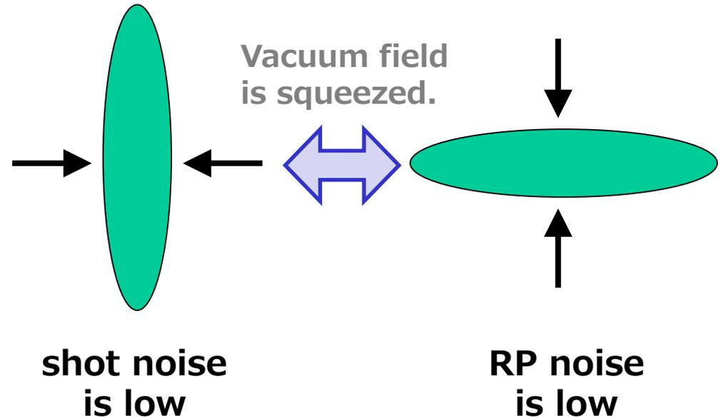
Sensitivity improves either at LF or HF according to the choice of the squeezing angle.
