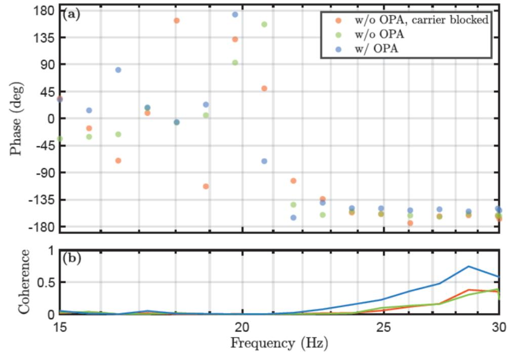
**Left: Without OPA, the optical spring was observed in phase of the transfer function.**
