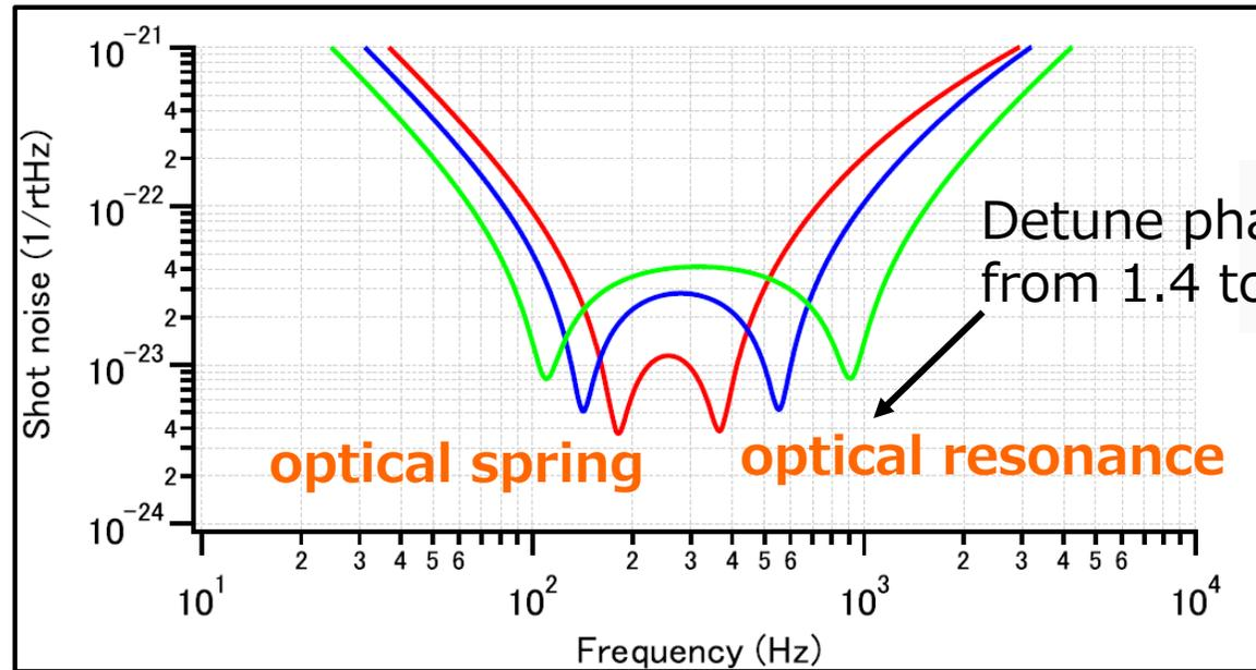
Optical spring  $\Omega \propto \sqrt{\frac{\sin 2\phi}{\left(r + \frac{1}{r}\right) - 2 \cos 2\phi}}$
