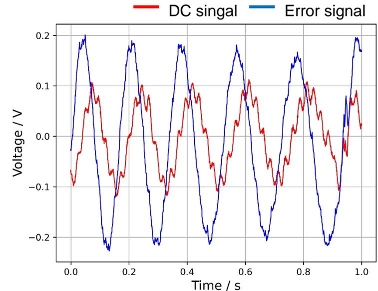
We use a secondary laser (20MHz different from main laser) and perform coherent-control method to obtain the error signal (demod at 40MHz).
