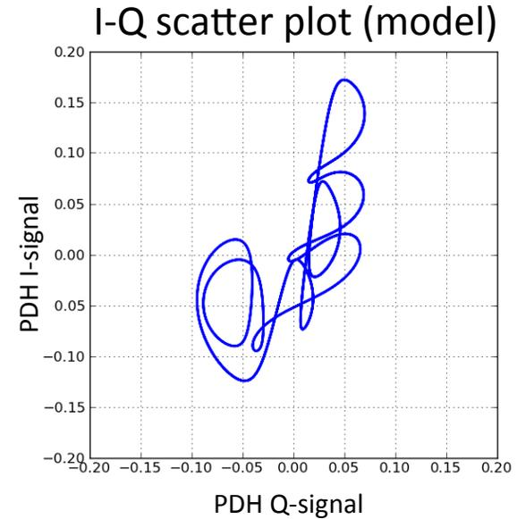
The model explained the distorted PDH signal due to HOM in the low finesse arm cavity for the green beam.
