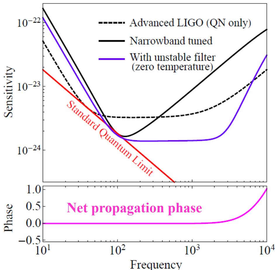
Sample parameters for optomechanical filter:
