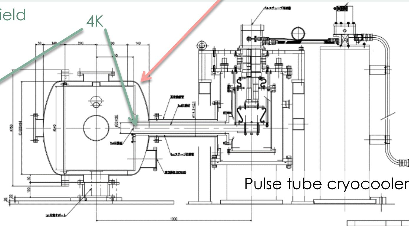
Pulse tube cryocooler
